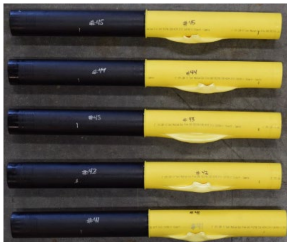
Pipe samples used during Teel's ASTM D2513 testing.
