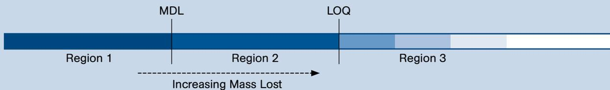
**Region 1:** Starting from the left at 0 mg, up to the MDL, the instrument can't reliably differentiate the amount of water lost from the measurement noise. Any result in this region is less than the instrument can detect.
