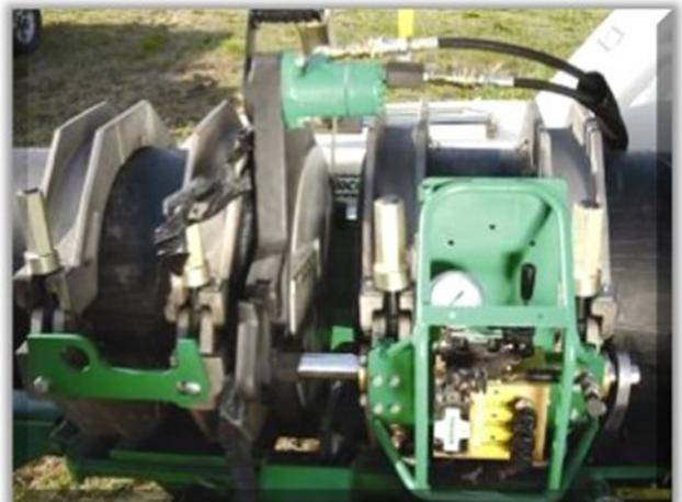
dry, lint-free cloth. **Do not touch the pipe ends with your hand or anything that could contaminate the pipe ends.**
