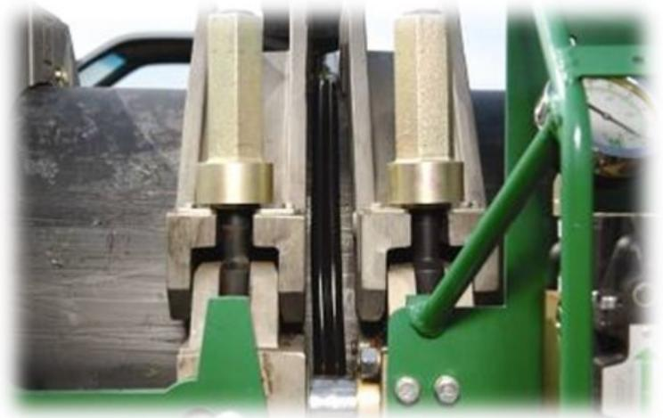
In Table 6 in Section 8 of the ASTM F2620 fusion standard, you will find the maximum time allowed to open the carriage, remove the heater and bring the pipe ends together for the fusion cycle. This depends on the pipes wall thickness.
