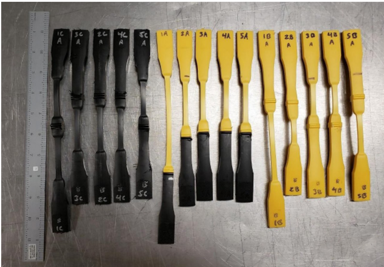
Figure 9: Teel's tensile properties test samples before and after testing
