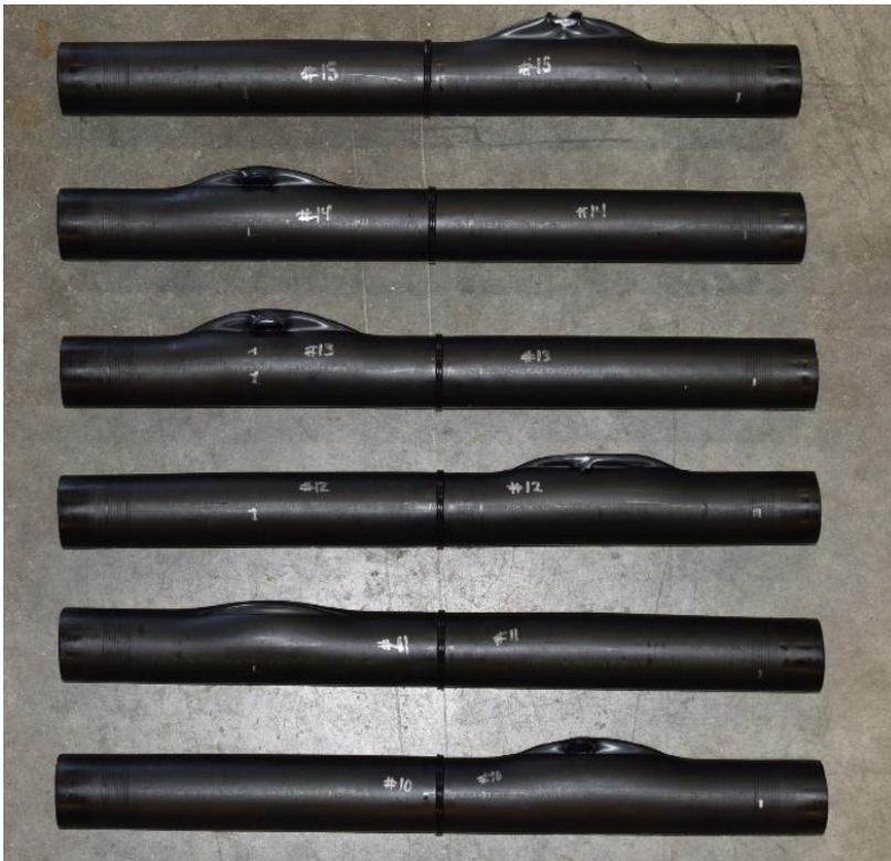
Figure 11: Teel's 2710 and 2708 quick burst test samples after testing
