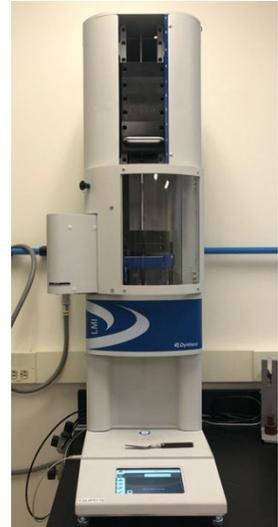
*Melt flow analysis testing device*
