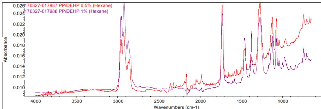
With this success, TAL was able to deliver a method to the customer for detecting DEHP at the specified levels.
