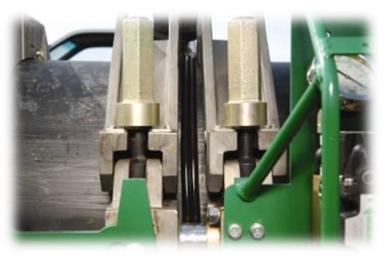
carriage by shifting the top carriage control valve to the center position. Remove the heater, inspect the pipe ends for the proper melt pattern (smooth with no marks or contamination). Then bring the pipe ends together by shifting the top carriage control valve to the left. The melt beads will roll back to the pipe surface. Maintain that hydraulic pressure for the entire cool cycle.
