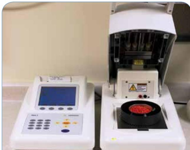
*Gravimetric moisture analyzers are commonly used to determine the percentage of moisture in resin. The instrument is essentially a sensitive balance contained within an oven.*
