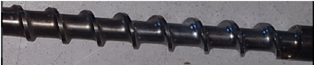
Figure 4: Feed section of a screw
